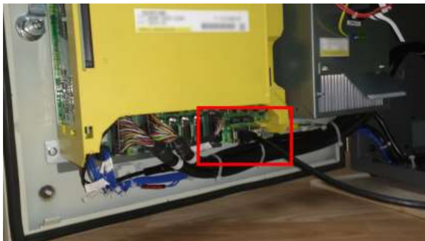
Ethernet port location on R-30iB Mate Cabinet controller (view of the opened controller door):
